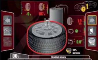
**iPos:** a special program for positioning the four wheels in the best possible way to guarantee the driver's comfort and safety.
