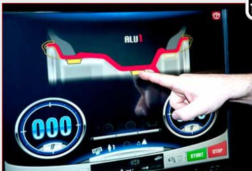
**Industrial 19" touchscreen monitor.** It resists dust, dirty or wet hands and is suitable for use with any type of glove. Quick and user-friendly graphic interface.
