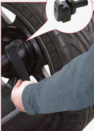
Adhesive counterweights can be applied very quickly by using the **laser pointer** at **6 o'clock** (laser line system) or by using the **weight holder clip** (optional) or **manually** at **12 o'clock**.
